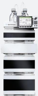
A low-dispersion UHPLC system, such as the Agilent 1290 Infinity II, is required for ultra-fast separations.
